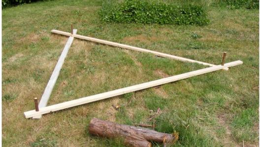
It's as simple as this. I just mark where the cuts need to be, along the ground braces, above and below. I will leave the tops of the uprights uncut for now. Eventually, they will have carved critter heads on them. Cutting where I have marked, at the ends of the uprights and ground brace will be my final step.
