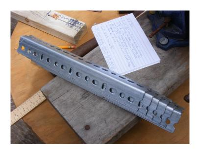
The use of carriage bolts with two pieces of angle iron for each join made a sturdy frame. But, for my next frame, I will use four longer pieces of flat iron on each join, and more carriage bolts. With the angle iron on 2" X 3", the holes could not be centered, and therefore not perfectly matched up with the opposite side.
