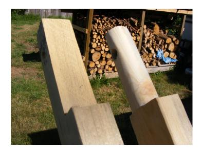
In order to fit the 12' 10" poles into my car, they had to be made in two pieces each. So, I needed a sturdy method of joining the two pieces together in order to raise the tent, once onsite. I have cut a 6' length of angle iron into six pieces, to create partial sleeves. A sleeve would have been good, but was beyond my area of skill.
